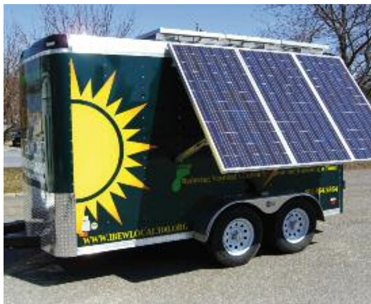
Local 300's mobile solar trailer features a one-kilowatt solar array.
